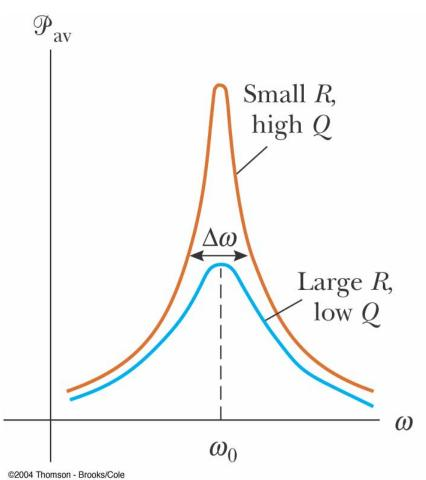
fo= fib It half power prequencies Power is half or current is to 8 max  $\frac{V}{\sqrt{2}R} = \sqrt{R^2 + 1}$ 72/2 or 2R2= 122+(x1-xc)2  $+2-xc=\pm R$ below fr,fi; Xc =Rabove fr XL-XC=R Ye-YL=R att, atte  $\frac{1}{\omega_{1C}} - \omega_{1L} = R$ at for W2L-L =R
